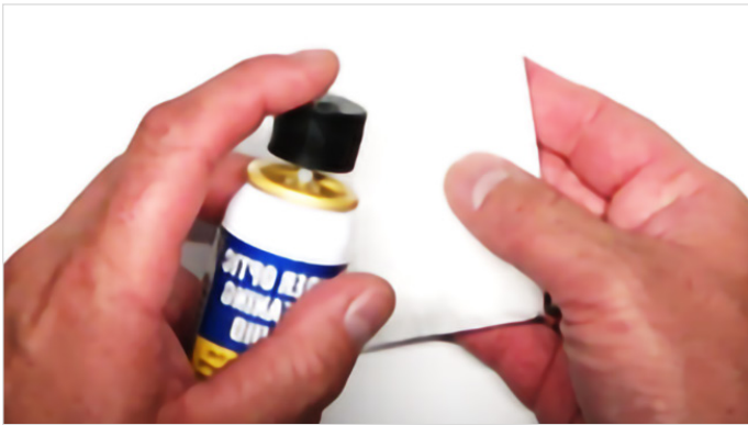
Figure 3: Apply Fiber Optic Cleaning Fluid
